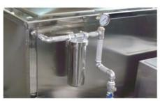
Filter. Filter element inside, can be replaced with new one
