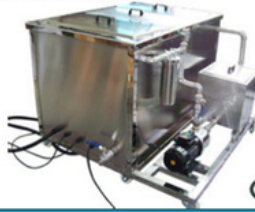
ultrasonic cleaner with filtration
