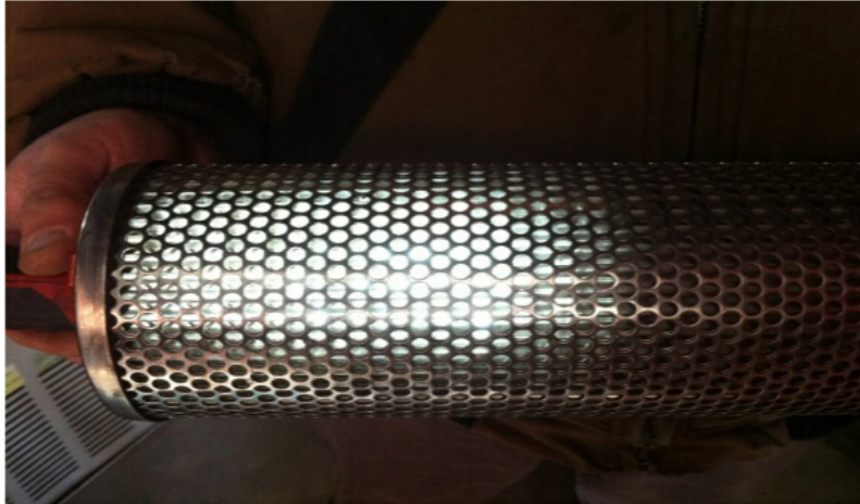
Cleaned oil filters with Light passing through
