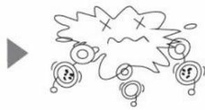
During the low pressure stage, millions of microscopic bubbles form and grow. This process is called "CAVITATION".
