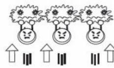
During the high pressure stage, the bubbles implode releasing enormous amounts of energy. They work in all directions, attacking surface and invading all recesses and openings.
