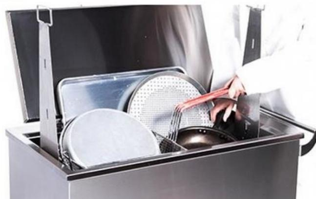
Remove the items from the tank, then simply rinse off any loose or softened carbon fragments.
