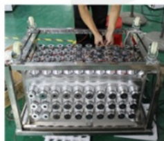
④ Transducer Installation
