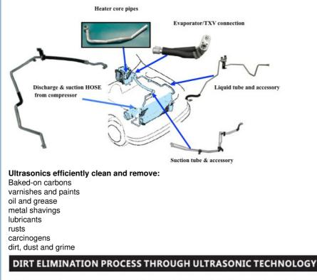
Cleaning effect will be much better if using the machine together with proper solvent.
