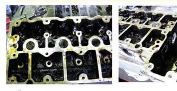
Engine block photo after cleaning by <u>Skymen</u> ultrasonic cleaner (from customer).
