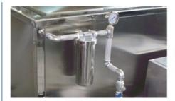
**Filter.** Filter element inside, can be replaced with new one
