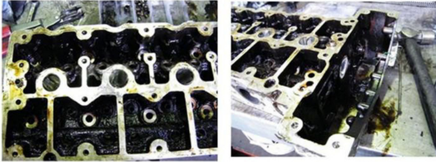
Engine block with heavy oil before cleaning (photo from customer workshop):
