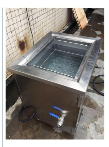
$2\ \text{Put}$  the clening items in, the cleaning items should fully immersed in the water. For oil removed, chemmicals is necessary.
