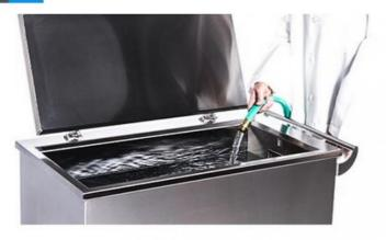
Fill the with (preferably hot) water to the 'Fill Line' marked on the inside, plug the tank into an electrical outlet, and switch ON
